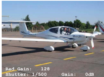
Typical on screen information. Example shows Red Gain is selected for variable adjustment. (simulated)
