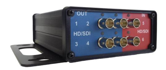
PanBox is a field deployable throw-down fibre optic transceiver that converts SD, HD or 3G video signals to one core (2+1 version) or 2 cores (4+2 version) of singlemode fibre cable. PanBox provides a robust housing with optional handle and colour codes the video inputs and outputs allowing ease of use. It also gives the units a more rugged field connector, in the Neutrik DUO or QUAD, and a 4 pin XLR power connector for a DC supply (included).
